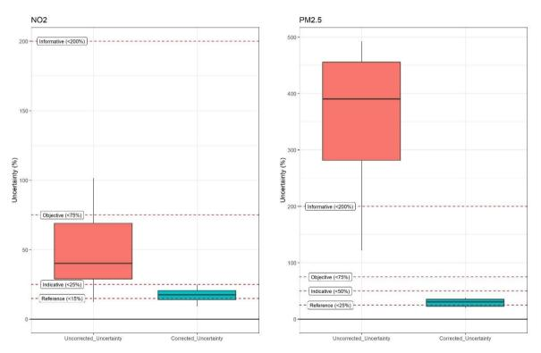
Figure 4 Comparison of node uncertainty before and after application of node specific correction algorithm.
