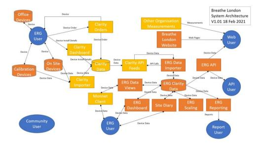
Figure 2 Data collection and data flow schematic
